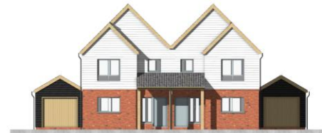
PROPOSED FRONT ELEVATION 1:100
