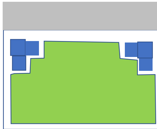
B: 8 x flats in two buildings with 2 per floor in each 2 storey building on 0.25ha = 32dph
