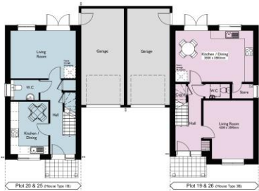
GROUND FLOOR PLAN (1:100)
